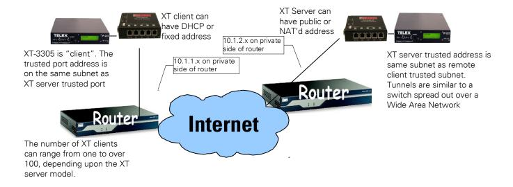
Telex IP addresses: 192.168.2.x at both ends of the link.
